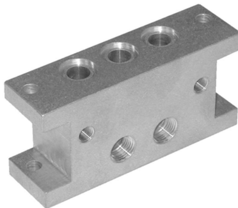
SM3 subplate showing 3/8" NPTF cylinder ports and 1/8" NPTF pilot ports located on the bottom of the subplate.
